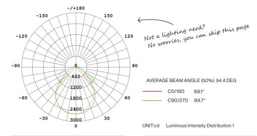
Lighting distribution angle refers to the spread of light emitted from a light source. It is an important factor to consider when selecting a fixture or bulb, as it affects the way it will illuminate an area. There are two main types of lighting distribution angles:
