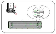
Release latches by pulling top of latch away from housing. Gently squeeze the buckle in and take out the PCB board (be careful not to touch the LEDs).
