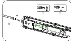
4. Separate the waterproof plug, and connect the input wire to the output wire of the power supply after passing through the plug and the outlet as shown in the figure.
