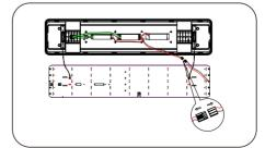
Disconnect the wire connecting the LED board and the driver to avoid unstable connection due to heavy suspension.
