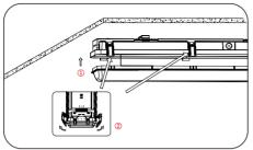
After align lens and bottom housing, turn off the luminaire. Secure lens to housing with lens latches.
