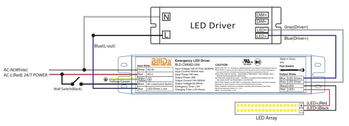
\* Note: During Emergency Mode, press test switch twice to cut off the emergency output and enter Shipping Mode.
