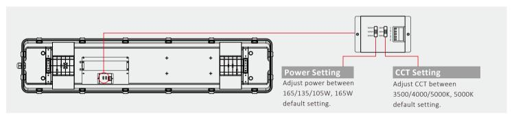
Note: Before Setting Power & CCT, release latches by pulling top of latch away from housing. Gently squeeze the buckle in and take out the PCB board (be careful not to touch the LEDs).
