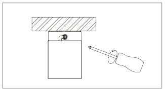
2. Fix the surface mount bracket on the ceiling with PA4\*30 screw.
