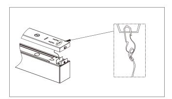
5. Fix screws on two side of the fixture.
