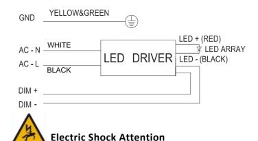
Ensure the power supply has been cut off before connecting the wire, and all wiring and installation of this product are required to be operated by professionals.
