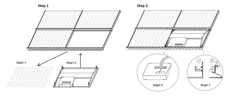
**Step 1:** Make sure of all the power is off before installing. Remove the one ceiling tile that you need to install light fixture on. Then place the light fixture on the T-bar carefully and make sure it is correctly in place and secure.
