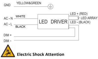
Ensure the power supply has been cut off before connecting the wire, and all wiring and installation of this product are required to be operated by professionals.
