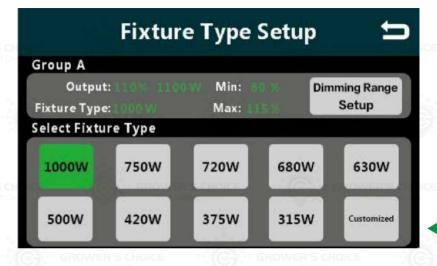
Touch "Fixture Type" to select fixture type and power levels.
