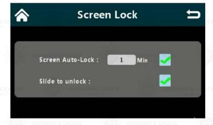
Touch "Screen Auto-Lock" to activate or deactivate screen lock and enter time before screen locks using the "min" option.
