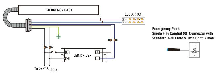
During Emergency Mode, press test switch twice to cut off the emergency output and enter shipping mode.
