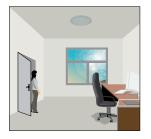
With sufficient natural light, the light does not switch on when a presence is detected.
