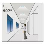
The light switches on at 100% when there movement detected.
