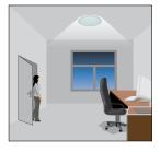
With insufficient natural light, the sensor switches on the light automatically when a presence is detected.
