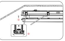
6. After align lens and bottom housing, turn off the luminaire. Secure lens to housing with lens latches.
