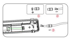
6. Separate the waterproof plug, and connect the input wire to output wire of the driver after passing through the plug and outlet as shown in the figure.
