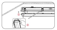
8. After align lens and bottom housing, turn off the luminaire. Secure lens to housing with lens latches.
