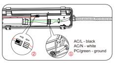
7. After the wire connection is completed, reconnect the wiring between the LED board and the driver.
