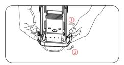
4. Release latches by pulling top of latch away from housing. Remove lens and set aside.
