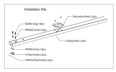
1.Drill Hole on the ceiling based on the Length of the fixture, fix the plastic anchor in the hole .
