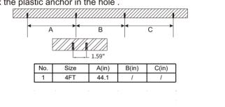
2.Fix the surface mount bracket on the ceiling with PA4\*30 screw.
