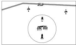
1. Locate drill holes for mounting brackets. Use hardware found in hardware kit. Mount bracket to surface.
