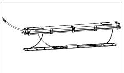
5. Connect power to driver as shown. (Flexible cord 6. Follow general wiring diagram. Make sure the supplied by installer)
