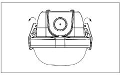
3. Release latches by pulling top of latch away from
