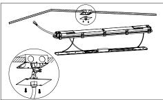
power supply is disconnected before installing.
