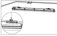
2. Secure mounting clips to housing recesses by firmly pressing them into place until both sides of the clip are secured.
