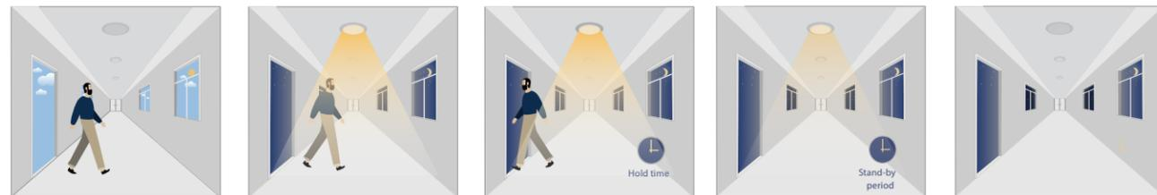
With sufficient daylight, the sensor keeps light OFF even motion gets detected
