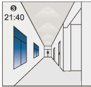
The light remains in dimming level at night.
