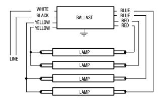
**INSTALL INSTRUCTIONS - ELECTRONIC BALLAST REQUIRED (UL TYPE A)**
