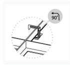
Turn brackets 90°. Hook should face outside edge of Ceiling Panel.
