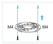
7. Tighten two M4 screws into expansion anchors to secure Adapter Plate.
