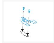
Use M3 screws to tighten Spring Bracket onto fixture relative to hole size (choice of 4", 5", 6").
