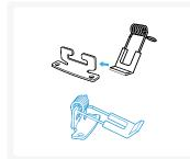
Fit Spring Clips onto Spring Brackets.
