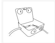
5. Feed supply wires through knockout. Secure with Romex connector (not included).
