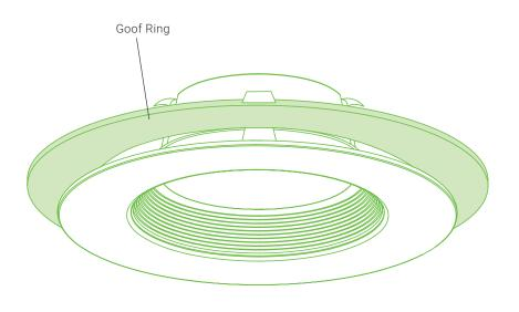
**Goof Ring is held in place by Recessed Light Fixture.**(Recessed Light Fixture not included)
