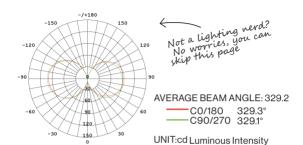
Lighting distribution angle refers to how light spread from light source and plays crucial role in choosing the right fixture or bulb. Symmetric lighting distribution emits light uniformly in all directions, forming a cone-shaped pattern that offers widespread illumination.
