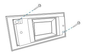
Secure the fixture in place by screwing the two screws through the holes on the fixture and into the mounting surface.
