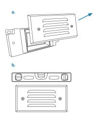
a. Begin by carefully removing the faceplate from the fixture.
