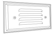
Reattach the faceplate, then use the two screws to secure it onto the fixture by fastening them through the holes on the cap.
