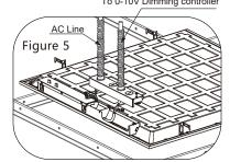
Plug in AC line to the LED Driver using 18-14AWG wire. When connecting 0-10V dimming controller, wire must run through a separate knockout hole equipped with an appropriate electrical fitting.
