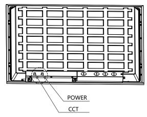
Double switch design can adjust power and CCT.
