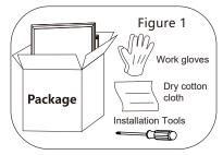
Carefully unpack unit and properly inspect for defects before installing. Wear work gloves to prevent dirt and oil from being transferred to the luminaire. If cleaning is needed and a dry cotton cloth. It is not recommended to use gloves, And prepare the installation tools.
