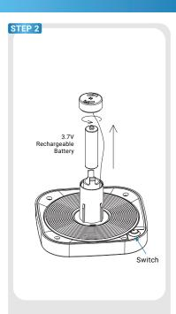
Press the button to select the preferred color tempterature. (To replace the rechargeable battery, unscrew the back cover counterclockwise)
