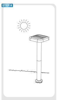
Note: Location should have clear access to sunlight and kept away from other sources of light that could interfere with sensor.
