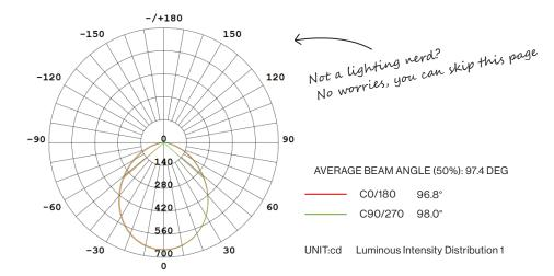
Lighting distribution angle refers to the spread of light emitted from a light source. It is an important factor to consider when selecting a fixture or bulb, as it affects the way it will illuminate an area. There are two main types of lighting distribution angles:
