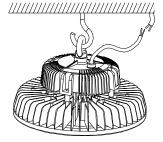
3. Connect the electrical cables; Brown-L, Blue-N, Yellow/Green-Ground. If using in wet locations, ensure all electrical connections and installation holes have a water tight seal.
