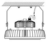
2. Connect the electrical cables. Brown-L, Blue-N, Yellow/Green-Ground. If using in wet locations, ensure all electrical connections and installation holes have a water tight seal.
