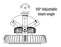
Adjust the bracket to the beam angle you need.
