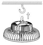
1. Drill a hole into the ceiling for the appropriate size hook (provided by installer).
