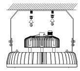
1. Attach the bracket to the mounting surface.
