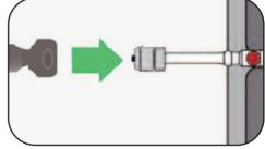
Connect the Direct Link<sup>™</sup> to the Input Assembly of the Stealth Watering System installed on the battery.
