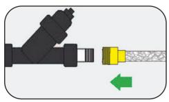
Attach the braided hose to the white male end of the sediment filter. Do not use more than 20 ft. of hose
