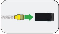
Attach the Pressure Regulator to the end of the red hose.
