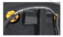
5. Connect the water feed line near the center of the battery onto an unused swivel connector port. Refer to the installation
