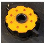
2. Insert the SPW valves into each battery cell by turning them in a clockwise direction.
