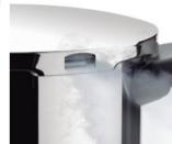
If both of the safety valves were not work, the rubber seal would expand, coming out of the groove of the lid, thus releasing the pressure from the cooker through the side away from the position of the user and leaving them safely protected. [2]
