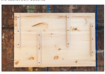
It is very important not to use glue to secure the ribs to the lid. Use screws only. If building a metalfree casket, then use glue and dowels to join the ribs to the casket, but do not use glue between the rib and the lid panel.
