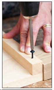
▲ Align screws in the center of the ribs. **DO NOT** over-tighten the screws!
