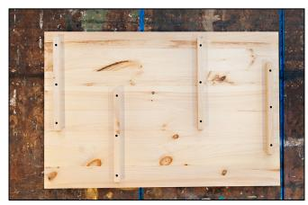
It is very important not to use glue to secure the ribs to the lid. Use screws only. If building a metalfree casket, then use glue and dowels to join the ribs to the casket, but do not use glue between the rib and the lid panel.
