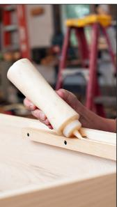
▲ Lay a bead of glue on each of the 8 ribs that will secure the floor.
