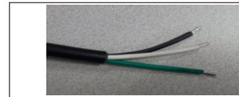
\*Please connect the input wire in correct way, white is ACN, black is ACL, GREEN is ground connection.
