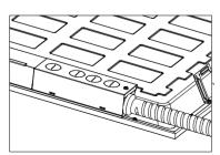
(3) Cover the driver box and tighten it with a screwdriver finish connection.
