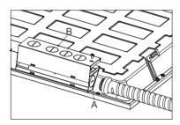
(1) Remove the knock-down hole on box by screwdriver (Part A),Remove screw and take out the driver cover (Part B)
