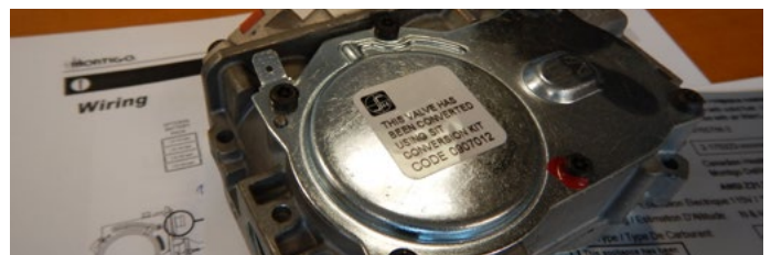
Figure 13.k Conversion label on valve
