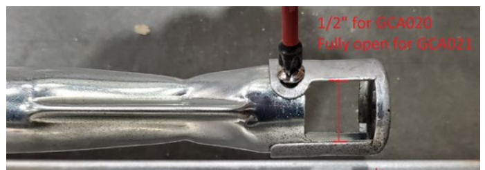
Figure 13.c primary air adjuster
