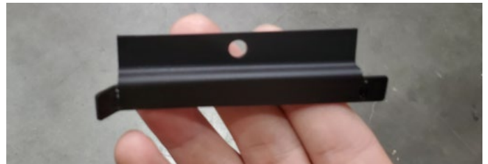
Figure 20.b Bend the left side tab
