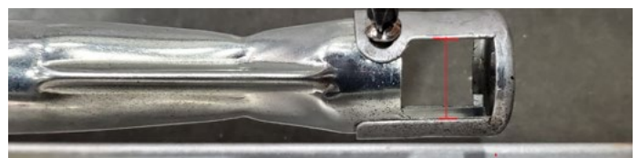
Figure 13.c primary air adjuster
