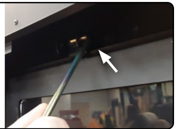
Figure 21.d Pull door latches
