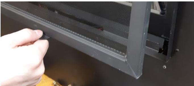
Figure 20.b Lift out the Retaining Tabs and screen
