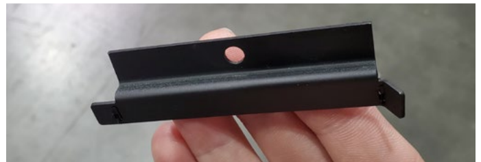
Figure 20.b Bend the right side tab
