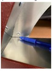
• Once the burner is removed you will need to remove the cover that is over the pilot assembly. (see photo below) Once this cover has been removed you will also need to remove the front top cover of the burner. (see Photo)
