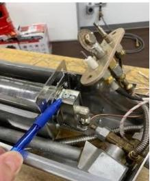
Now you can remove the air shutter to access the burner orifice. (see photo) With air shutter removed you can remove the #230 burner orifice and install the #400 that came with the oven. You will need an 11mm wrench or a 7/16" wrench to do this.
