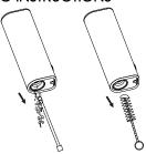
3. Use the cleaning brush to sweep the remaining residue from chamber
