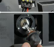
• For H10, 9005, 9006, H11, H9, H8, 9012, 880, PSX26W, H13, carefully, inserts the bulb into the headlight housing and secures it by twisting it into place. Once the bulb is secured, connect the factory connector to the LED driver.
