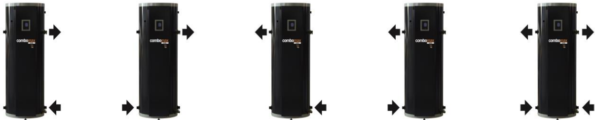
Figure 1: Possible installation configurations
