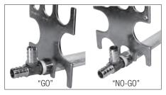
Joints that do not pass the gauge check must be cut out and replaced. DO NOT RECRIMP (Double Crimp) THE SAME FITTING.
