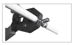
Check each crimped ring with the proper gauge. Slip gauge squarely over the crimped ring. Check in at least two positions. The "GO" portion of the gauge should slip over the ring. If not, the ring is under crimped. For gauges with "NO-GO" dimensions, the "NO-GO" gauge should not slip over the ring.
