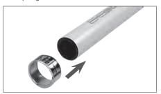
Insert a PEX fitting into tube up to the fitting shoulder and position the crimp ring 1/8" to 1/4" from end of pipe. To prevent ring from moving, squeeze the ring slightly with your fingers or a pair of pliers.
