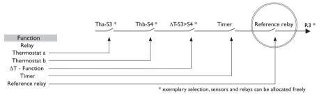
Reference relay Ref. relay 1 Ref. relay 2 Ref. relay 1 Ref. relay 3 Ref. relay 5 Ref. relay 3 If more than one function Ref. relay 2 Ref. relay 4 Ref. relay 4 block has been activated. Ref. relay 5 relays of numerically higher function blocks may not be used as reference relays. 1. in parallel (OR) 2. in series (AND)
