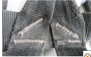
• Damaged safety stitching
