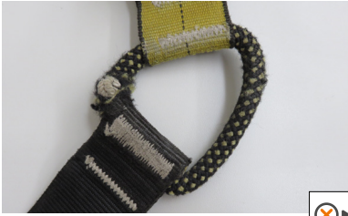
• Damaged attachment point
