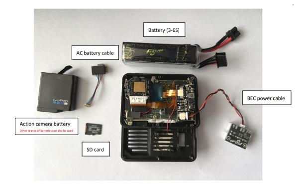
6. Insert SD card, connect AC battery and BEC power.
