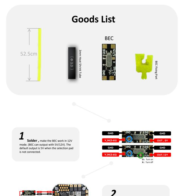
**Remove** the tape behind the LED strip to expose the pad . Solder the LED strip and BEC to the FC
