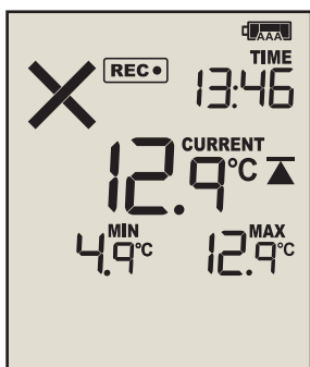
Recording - Upper Alarm.
