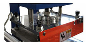
Four-point balance adjustment
