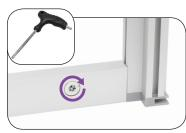
**e.** Use Torx Key to tighten and secure connection.
