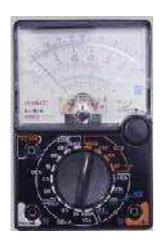
Set the meter in the Ohm settings  $(\Omega)$ . Place one lead of the meter to one of the wires from the controller, while the other end to the corresponding color in the pedal. Plastic insulator covers the clips attached to the controller, you have to push it down before doing the procedure below.
