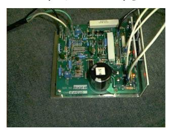
The next step will include a couple of things. There are two screws that hold the controller in place. This can be seen on the side of the frame. Before you loosen the screws, first take the wires out, with the use of needle nose pliers or simply by just pulling the connector by hand. Don't worry about which goes to which, a schematic and step by step procedure will be given later to put the controller back into place.
