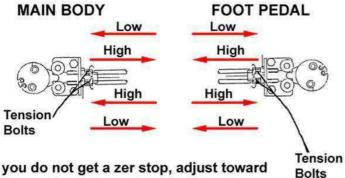
If you do not get a zer stop, adjust toward Low position. For a higher RPM, adjust to High position either at the foot control box or at the body control box.
