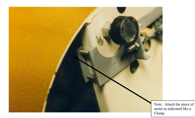
B. Remove Remote Control and Attach Fixed Pedal
