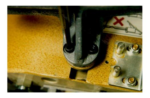
6. Attach lever pedal and tighten 2 socket bolts on lever pedal.
