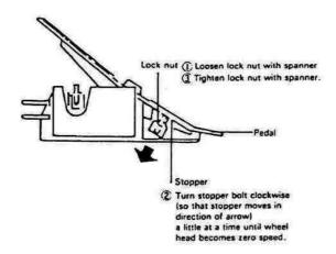
If wheel head continues to rotate after making above adjustment, wire tension adjustment is neccessary. Follow instruction  $\Theta$
